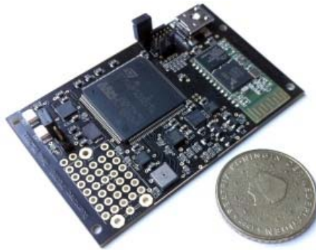
Figure 1: Inertial Measurement Unit “CCASS IMU200” (Münter, 2011)
